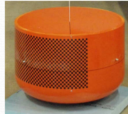
Cylinder in the wave tank during experiments (left), discretization for the numerical evaluation (middle), scaled-down physical model (right)
